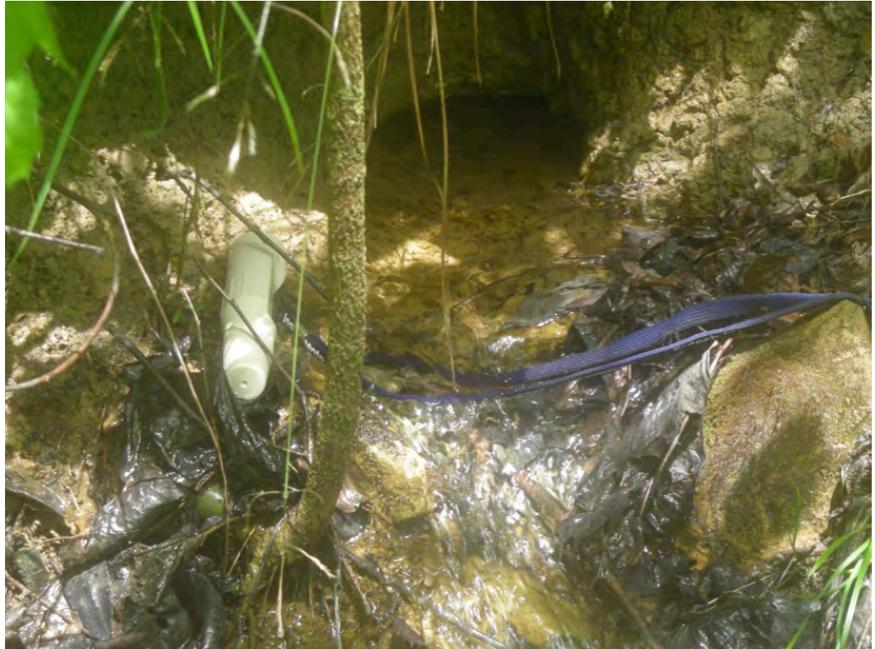
This photo shows a conductivity meter resting in a flow of water coming from a new hole, or blowout, in the side of the mountain.
