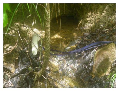
This photo shows a conductivity meter resting in a flow of water coming from a new hole, or blowout, in the side of the mountain.
